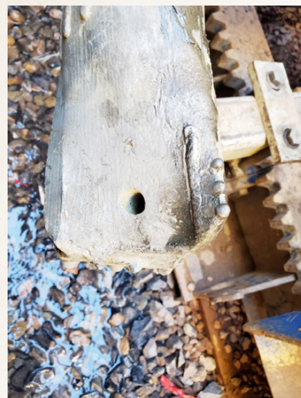
Figure 6B. The Trihawk IV bit following the first 160 feet of installation
