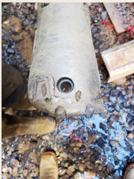
Figure 6B. The Trihawk IV bit following the first 160 feet of installation
