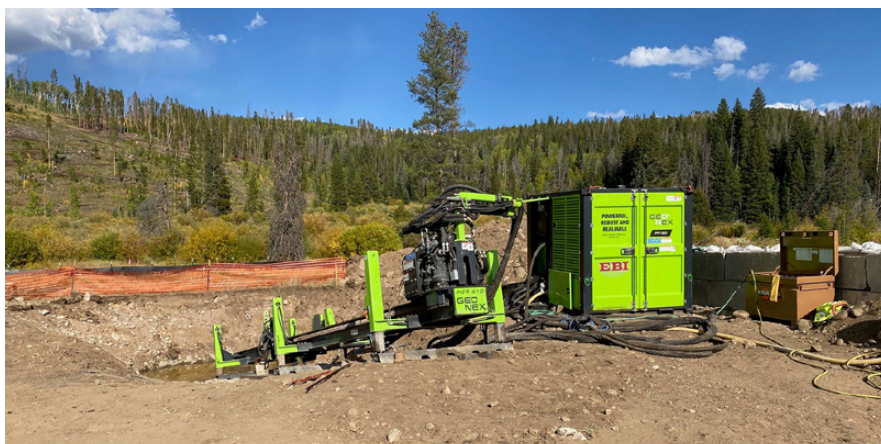
System consists of 3 main components, a drill machine, hydraulic power pack, and air compressors
