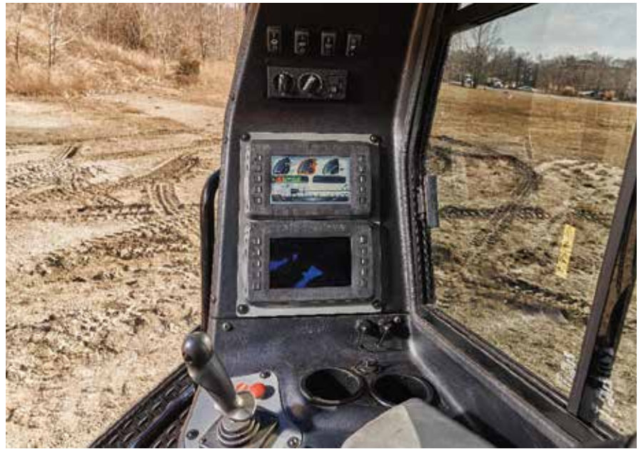
Figure 2. The integrated display of the Ditch Witch AT32 identifies service points and service intervals for operators.
