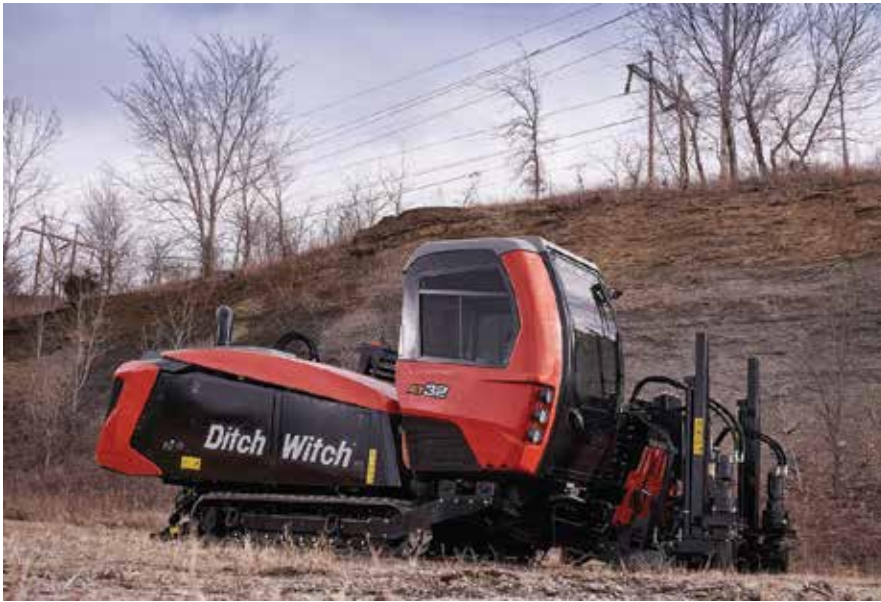
Figure 3. The JTAT32 is a mid-size directional drill designed to offer up to 4,200 ft-lbs (5,694.4 Nms) of outer rotational torque and 1,200 ft-lbs (1,627 Nms) of inner rotational torque.
