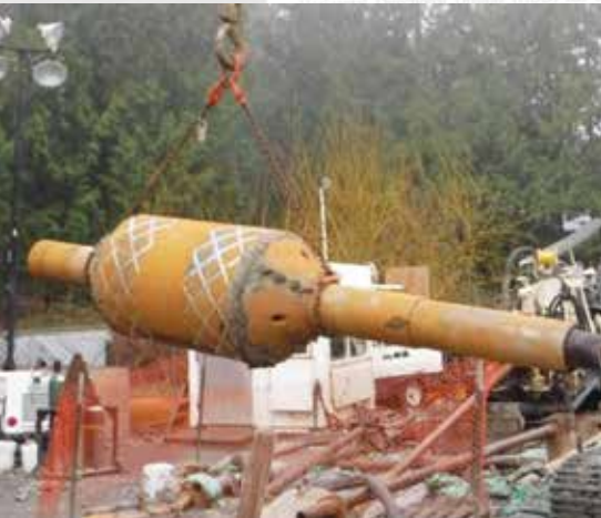
Figure 8. Typical barrel reamer used for a Swab Pass after the completion of reaming to the final diameter
