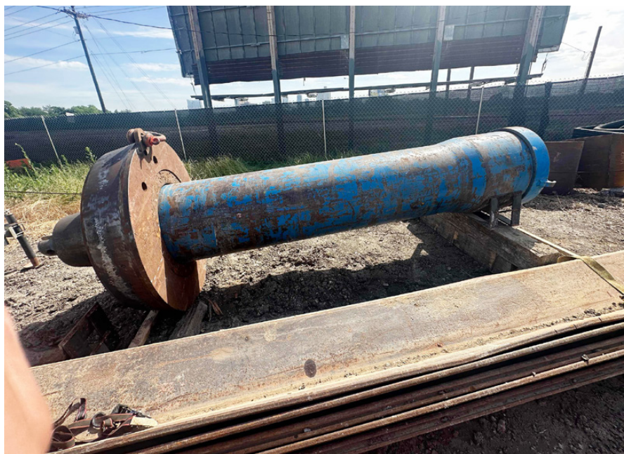
Iowa Trenchless used a Grundroram Pipe Ramming system from TT Technologies to install the Conductor Barrel Casings. Shown: Pipe rammer with ramming gear attached
