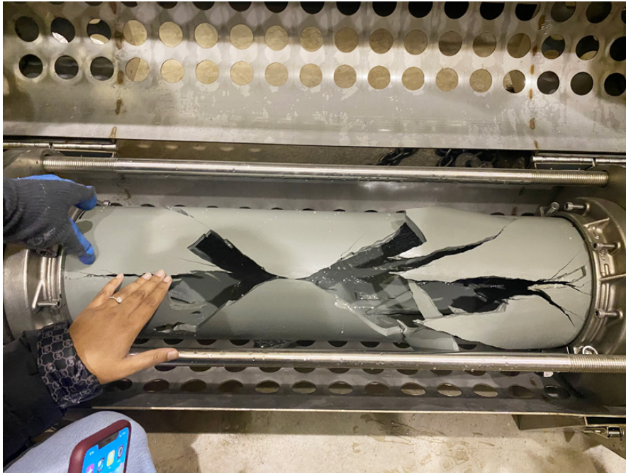
Figure 4: Hydrostatic Burst Test
