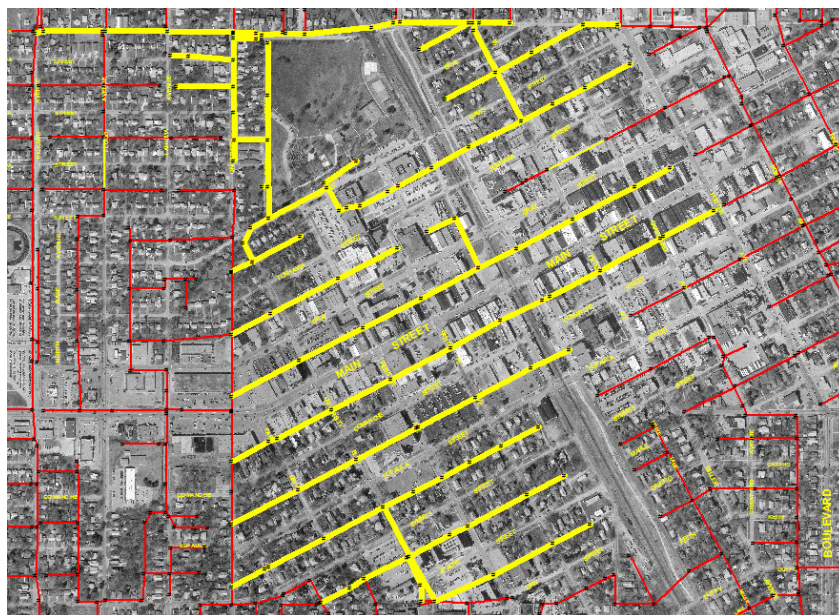
Figure 4: Year one covers more than 31,000 linear feet in the core Norman area that drains into the Imhoff Creek Basin
