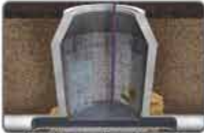
Curtain grouting with wand
