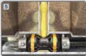
Lateral packer injecting grout
